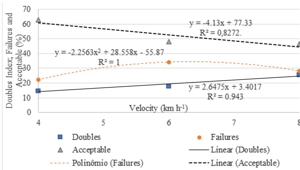
**Figure 5.** Regression analysis of variables: doubles, failures and acceptable in soybean crop with seed treatment “On farm” in T1 at speeds V1; V2 and V3 (4; 6 and 8 km h<sup>-1</sup>).
