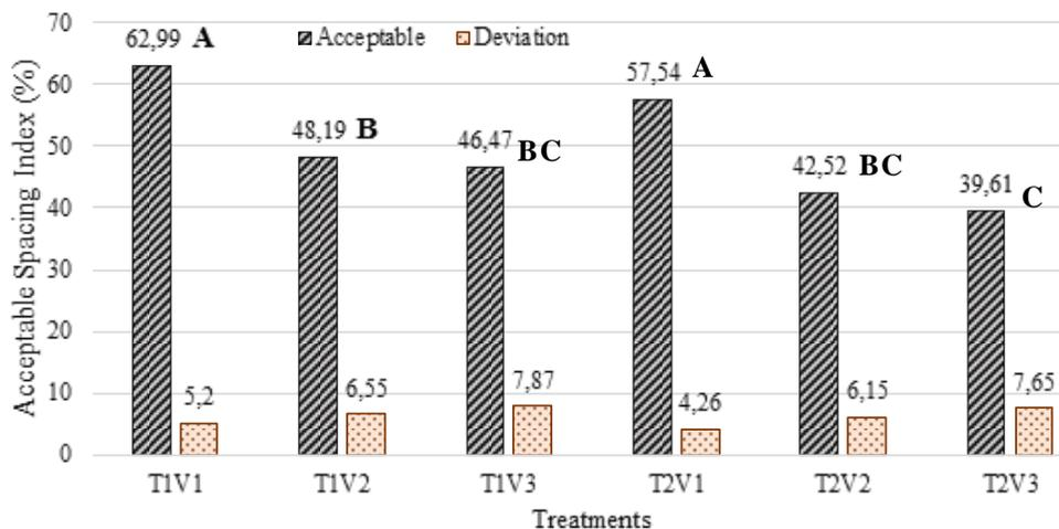
**Figure 4.** Soybean acceptable spacing index as a function of T1 and T2 seed treatments and V1 speeds; V2 and V3 (4; 6 and 8km h<sup>-1</sup>) with respective standard deviations (SD). \*Equal letter averages do not differ statistically between treatments according to the Tukey test at 5% probability. (n=12; F=8.89; p=0.000)
