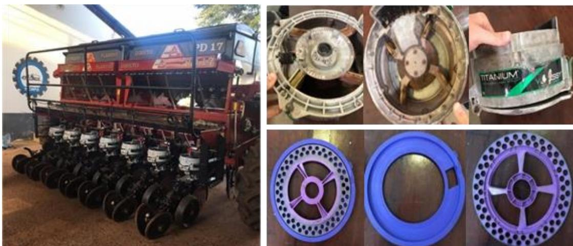
**Figure 1.** Seeder and dosing mechanisms used in the experiment.
