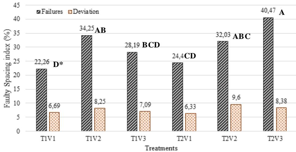
**Figure 2.** Soybean faulty spacing index as a function of T1 and T2 seed treatments and V1 velocities; V2 and V3 (4; 6 and 8km h<sup>-1</sup>) with respective standard deviations (SD). \*Equal letter averages do not differ statistically between treatments according to the Tukey test at 5% probability. (n=12; F=8.89; p<0.005).
