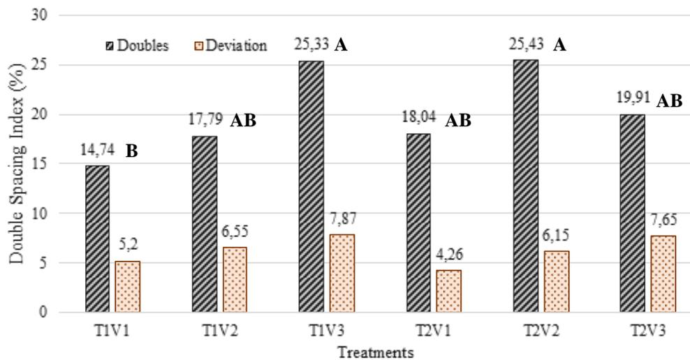
**Figure 3.** Soybean double spacing index as a function of T1 and T2 seed treatments and V1 velocities; V2 and V3 (4; 6 and 8km h<sup>-1</sup>) with respective standard deviations (SD). \*Equal letter averages do not differ statistically between treatments according to Tukey's test at 5% probability. (n=12; F=8.89; p=0.000).
