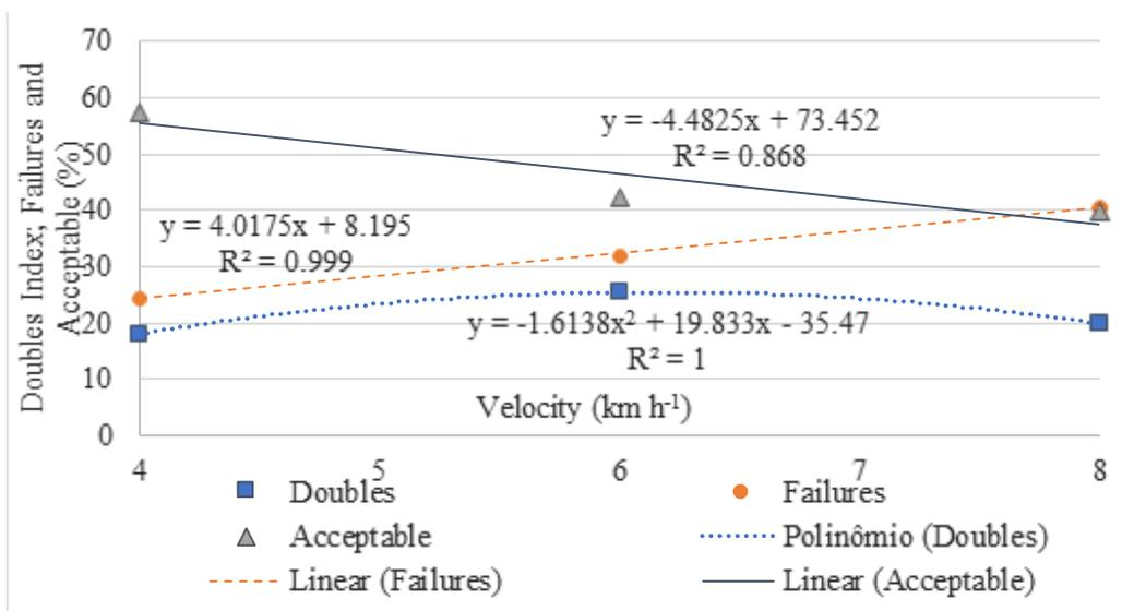
**Figure 6.** Regression analysis of variables: doubles; failures and acceptable in soybean crop with seed treatment “On farm” in T2 at V1 speeds; V2 and V3 (4; 6 and 8 km h<sup>-1</sup>).
