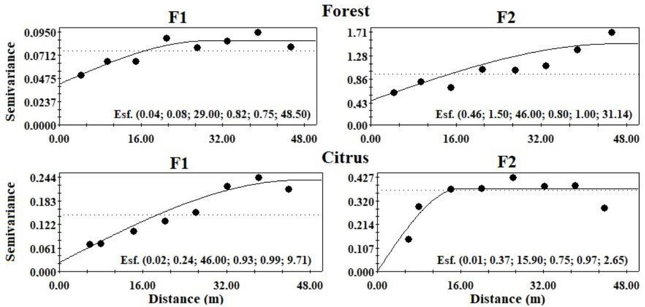
**Figure 5.** Experimental semivariograms fitted to principal component score values for citrus and forest areas in Southern Rondônia, Brazil. The values in parentheses are, respectively, Sph. = spherical; nugget effect; plateau; reach; R<sup>2</sup>; cross-validation; and DSD. Source: Author, 2023.
